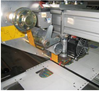
Stepper motor cylinder system for used foil rewinding.
