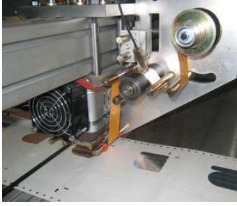
Hologram foil feeding system and stretching check at the printing unit.
